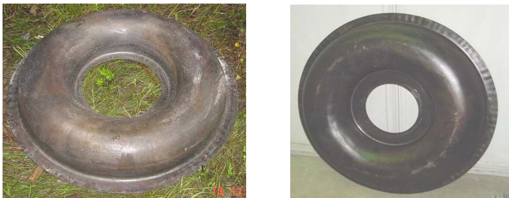
Fig. 19 Annular part after the deep drawing and calibration
