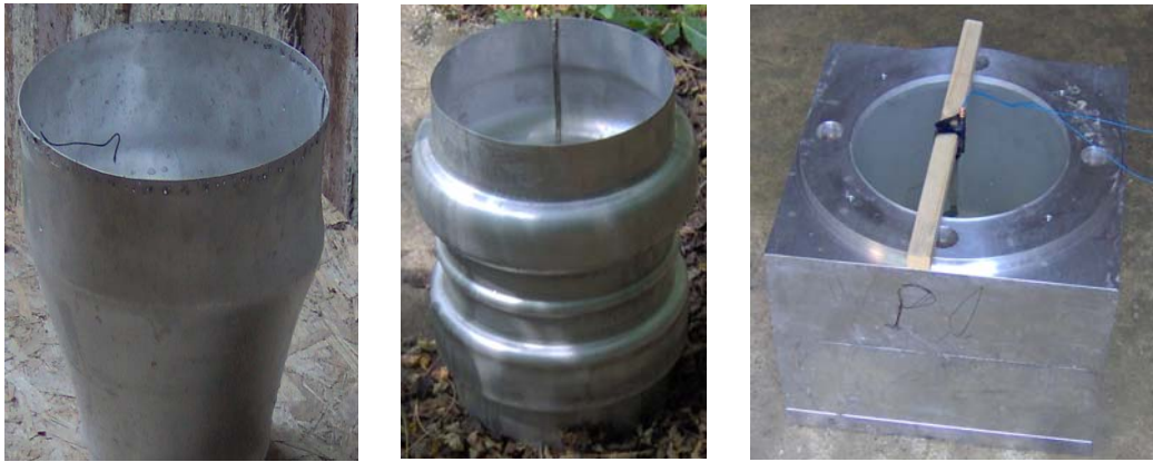
Fig. 17 Corrugated joint: half-finished product, manufactured part, explosion device.
