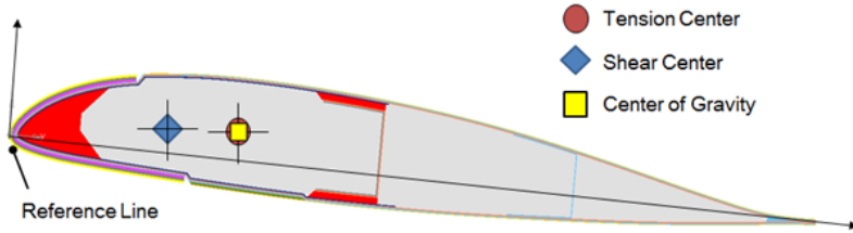
Fig. 5 The configuration and coordinates of cross-section of helicopter rotor blade
