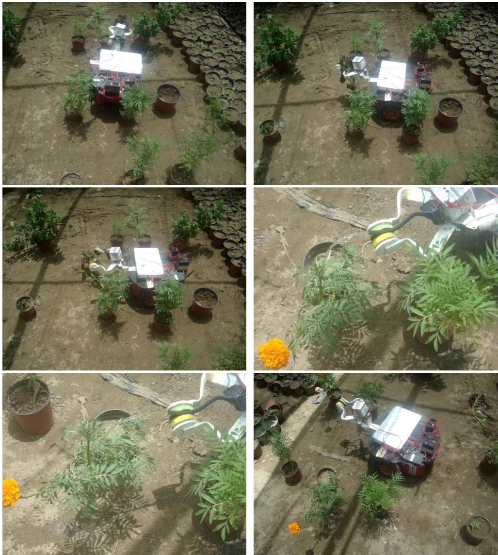
Fig. 15 Some of treatment for the sick plant (yellow) and elimination of weed (red)
