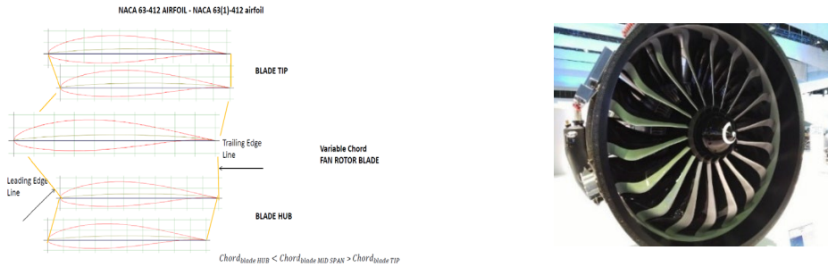
(a) – Generating the Airfoil Surface in case of a Fan Rotor Blade, with variable chord Blade spanwise and multiple sweep effect, similar to GE CFM LEAP-X Turbofan Engine's Fan Blade
