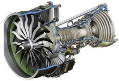
(b) – General Electric GE9X Turbofan Engine, cutaway, https://airpowerasia.com/2020/12/20/major-aircraft-turbofan-engine-manufacturers/
