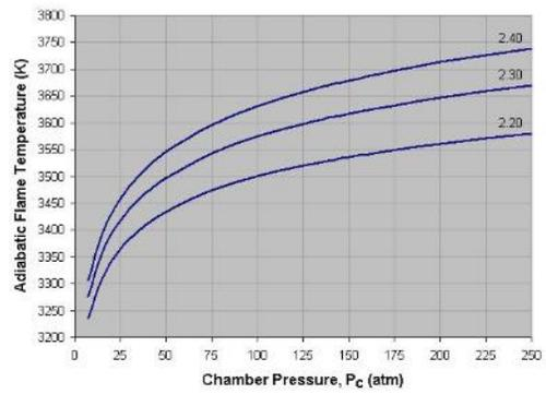
Fig. 2 - Adiabatic flame temperature, LOX-K, [1]
