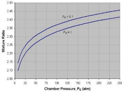
Fig. 1 - Optimum mixture ratio, LOX-K, [1]
