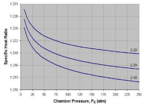
Fig. 4 - Specific Heat Ratio, LOX-K, [1]
