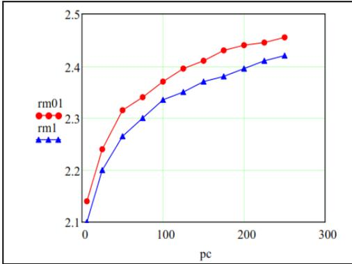
Fig. 9 – Input data for LOX-K: Mixture ratio, chamber pressure, nozzle exit pressure =1 [atm] - blue contour, and = 0.1 [atm] – red contour
