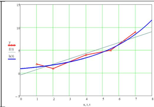
Fig. 8 – Least squares approximation, linear versus non-linear regression, [13,14]
