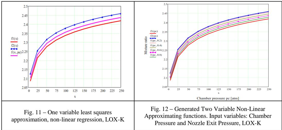
The two-variable non-linear approximation (17), (28) was used to generate the intermediate functions for other different values of the nozzle exit pressure, e.g. 0.2, 0.4, 0.6 and 0.8 [atm], which were depicted in Fig. 12.
