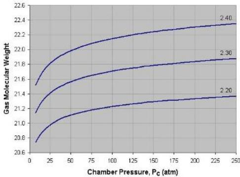
Fig. 3 - Gas Molecular Weight, LOX-K, [1]
