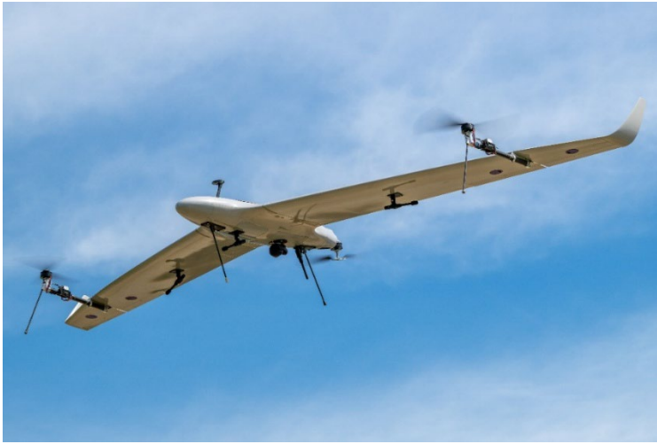
Figure 1 - Investigated hybrid flying-wing UAV during an experimental VTOL flight
