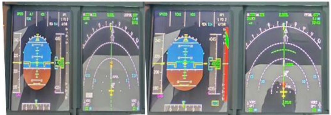
Fig. 8 TCAS is activated by distance < 5 NM
