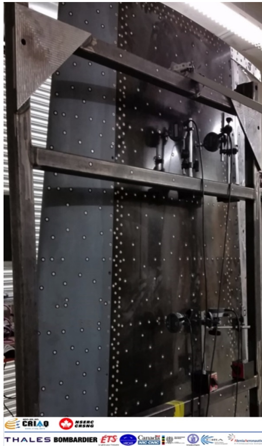
Fig. 3 Airfoil validation by dial indicators
