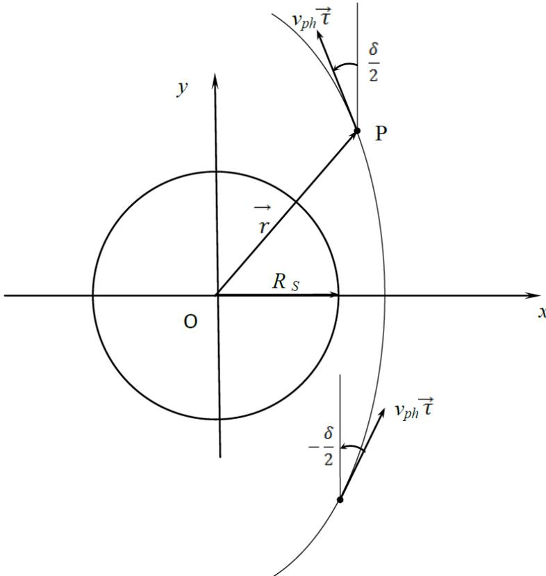
Fig. 2 The passing of a photon near the Sun;  $R_s$  - sun radius;  $\delta$  - the deviation angle;  $v_{ph}$  - the speed of photon ;  $\vec{\tau}$  - the tangent unit vector.
