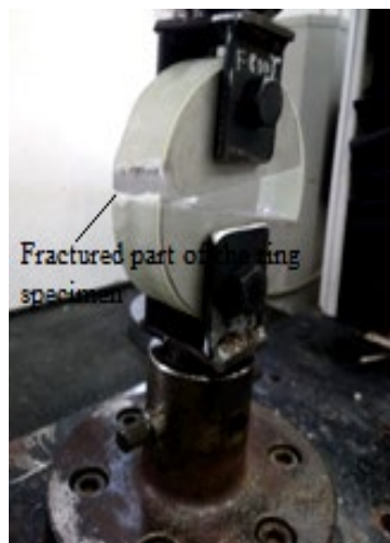
Figure 7: Fractured part of the test specimen after hoop tensile test
