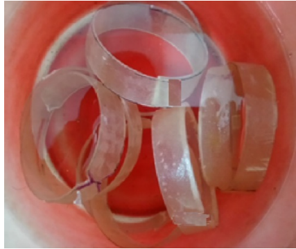
Figure 3: Submersion of E-glass and S-glass fiber reinforced epoxy rings under artificial seawater
