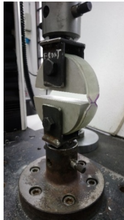
Figure 4: Split disk test setup according to ASTM D2290 on the UTM machine
