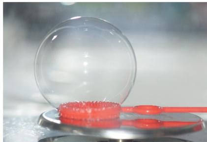
Fig. 4 – Set-up for weighting the bubbles. The photographs were used to measure the diameter of each weighted bubble
