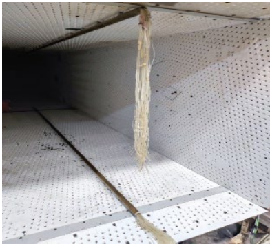
Fig. 4 – Tubular pressure probes placed on the top and bottom walls of the test section
