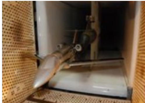
Fig. 2 – INCAS perforated wall test section
