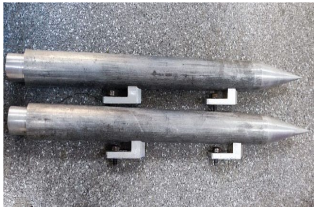
Fig. 5 – The tip of the pressure probes
