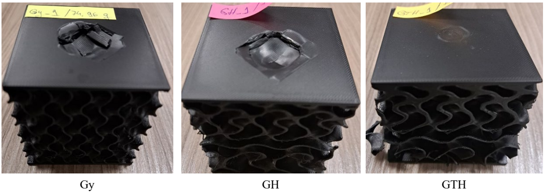
Fig. 8 - Damage morphology and crater depth after impact. GH exhibits the shallowest crater, while GTH retains the upper face without perforation but undergoes extensive global deformation
