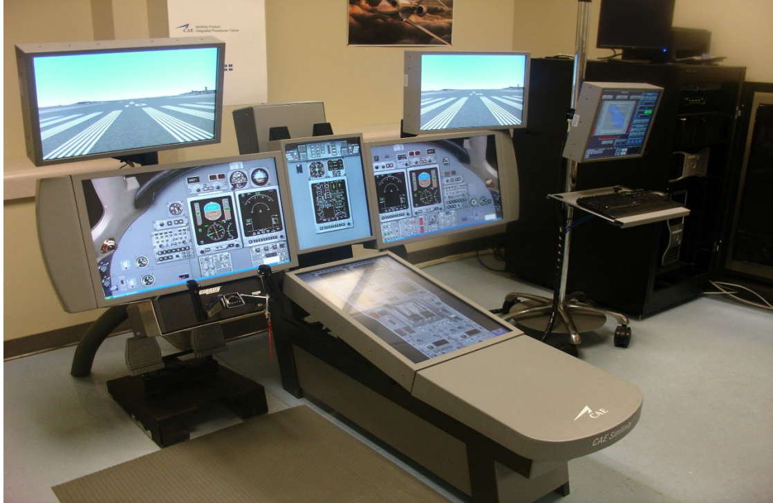
Research Aircraft Flight Simulator (RAFS) for the Cessna Citation X Business Aircraft (developed in collaboration with CAE and Cessna)
