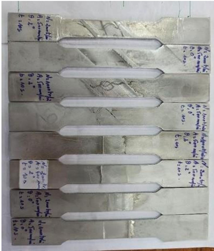
Fig. 3 – Cutting of samples on welded plates according to ASTM E8 M 04 (Dimensions in mm)
