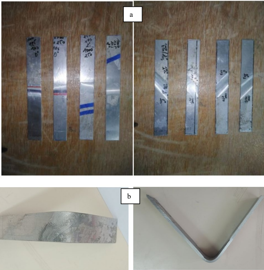
Fig. 9 – a): Bending specimens; b): Photographic view of bend samples after the experiment
