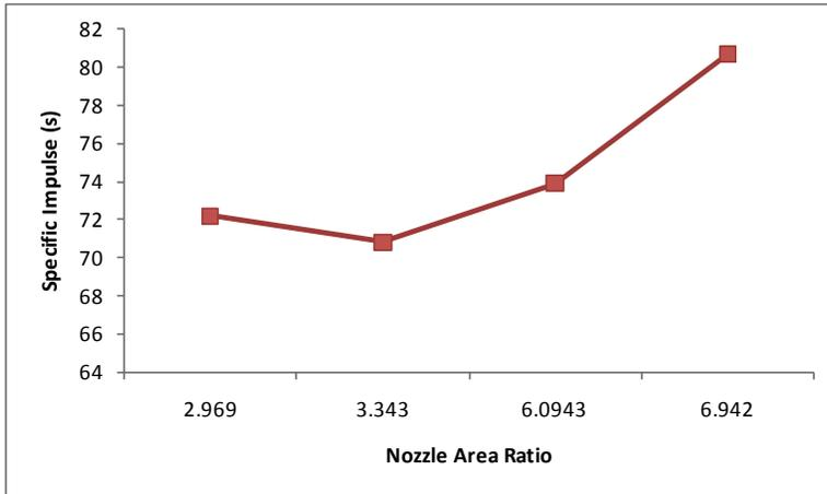
Fig. 7 Specific impulse variation with area ratio for Bell shaped nozzles
