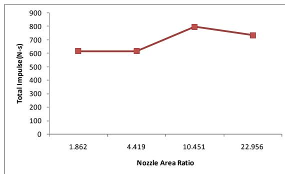
Fig. 11 Total impulse variation with area ratio for divergent nozzles
