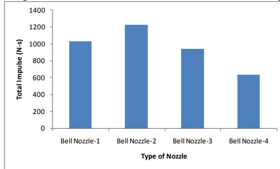
Fig. 10 Total impulse for Bell Shaped nozzles
