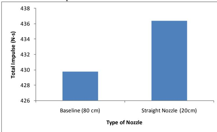
Fig. 8 Total impulse for the baseline engine and straight nozzle
