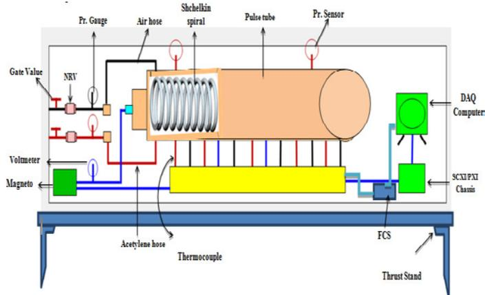
Fig. 1 Simplified layout of a basic PDE system
