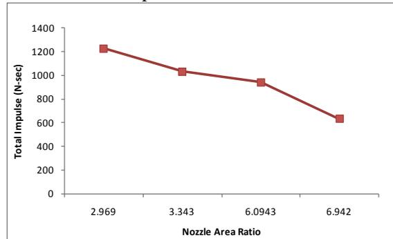
Fig. 12 Total impulse variation with area ratio for Bell shaped nozzles
