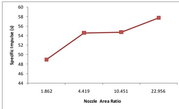
Fig. 6 Specific impulse variation with area ratio for divergent nozzles
