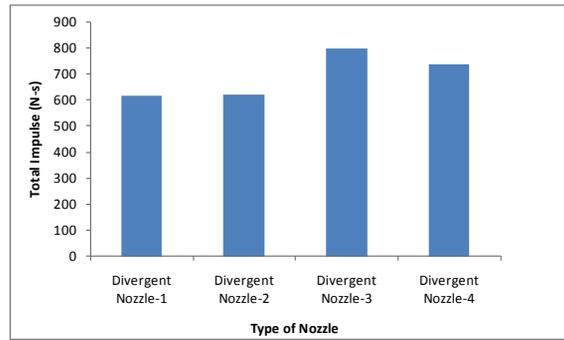
Fig. 9 Total impulse for divergent nozzles
