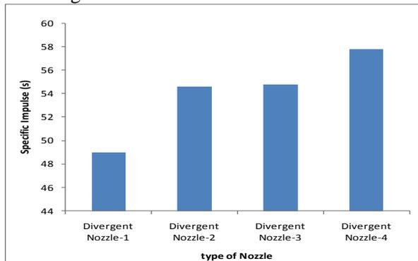
Fig. 4 Specific impulse for divergent nozzles
