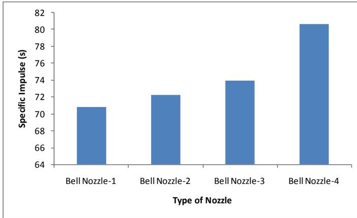
Fig. 5 Specific impulse for Bell shaped nozzles
