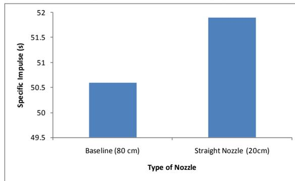
Fig. 3 Specific impulse for baseline engine and straight nozzle
