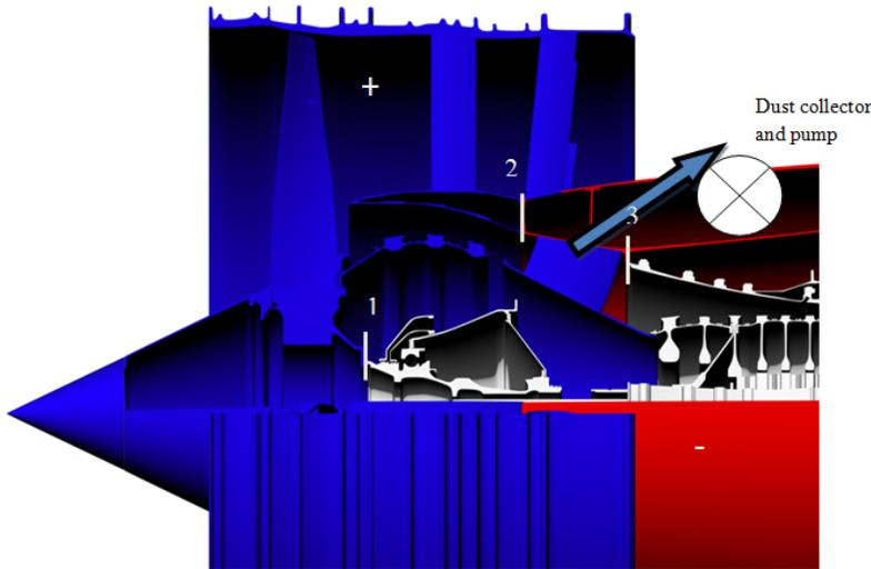
Fig. 2 Locations of retrofitting for Electrostatic Core Filtering System (Insulator gasket, washers and bolts 1, 2, 3)
