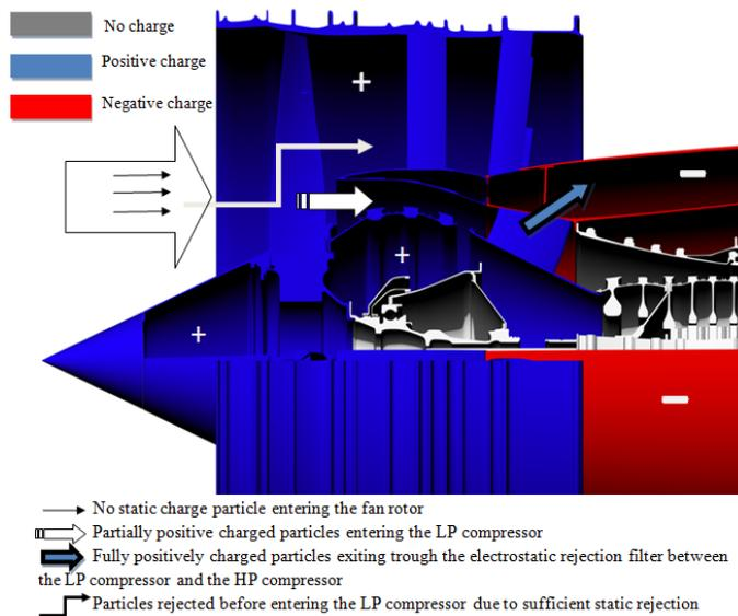
Fig. 1 The cutaway of a CFM 56-7 with polarization scheme and aerosol expected trajectories (blades are not shown in order to simplify the view)
