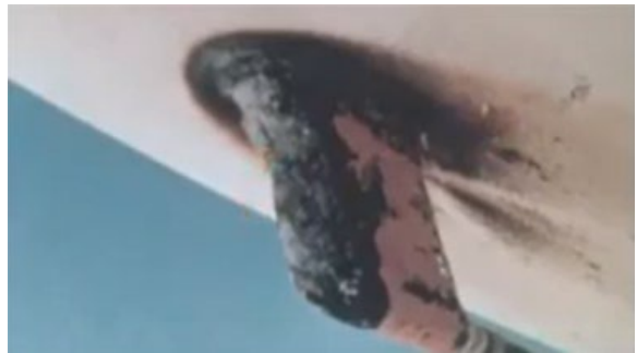
b) aerothermal heating of UHF Antenna (blunt fin SBLI)
