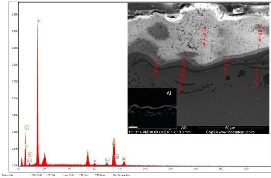
Fig. 9 Specimen microstructure after 25 h of testing (1 cycle)
