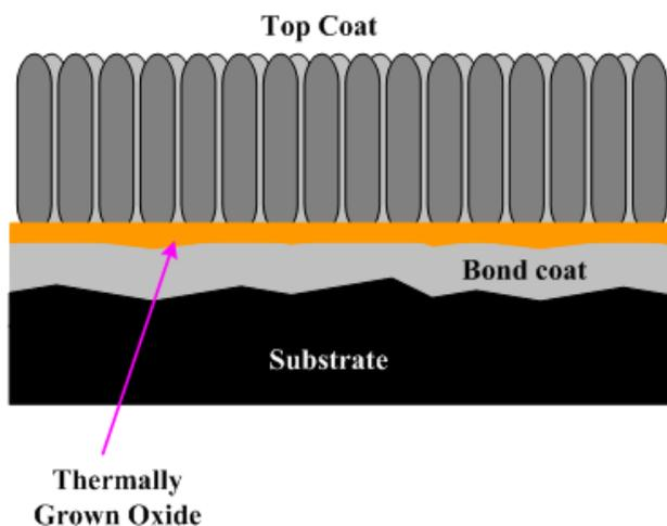
Fig. 1 Construction of thermal barrier coatings [5]
