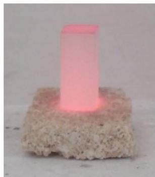
Fig. 7 The sample after the first test (25 h in furnace)
