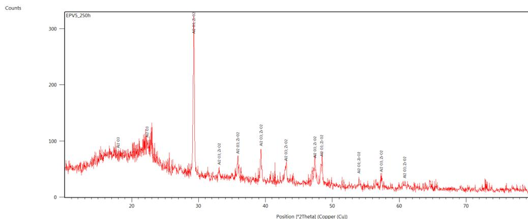
Fig. 13 X-Ray Diffraction of thermal barrier coating MeCrAlY / ZrO<sub>2</sub>8%Y<sub>2</sub>O<sub>3</sub> of sample after 250 h testing (10 cycles) at 1000°C
