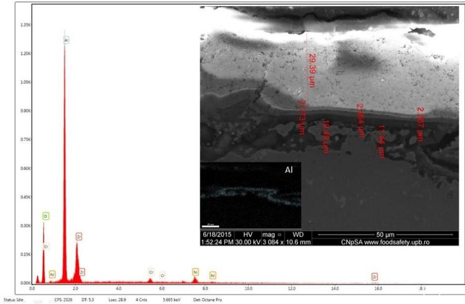
Fig. 11 Specimen microstructure after 200 h of testing (8 cycles)
