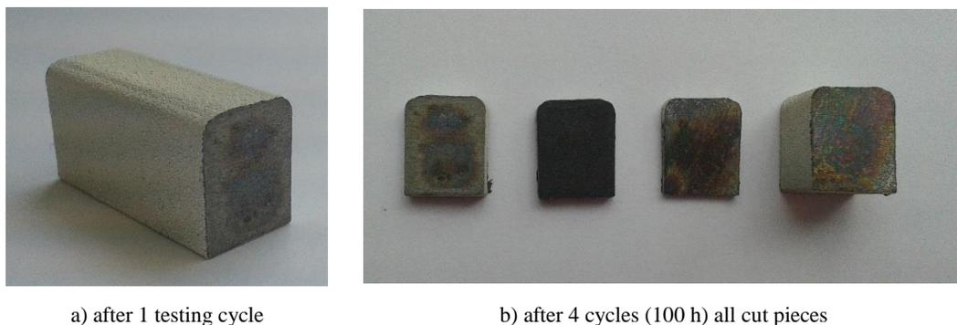
Fig. 8 Specimen 1 prepared for the first test at 1000°C
