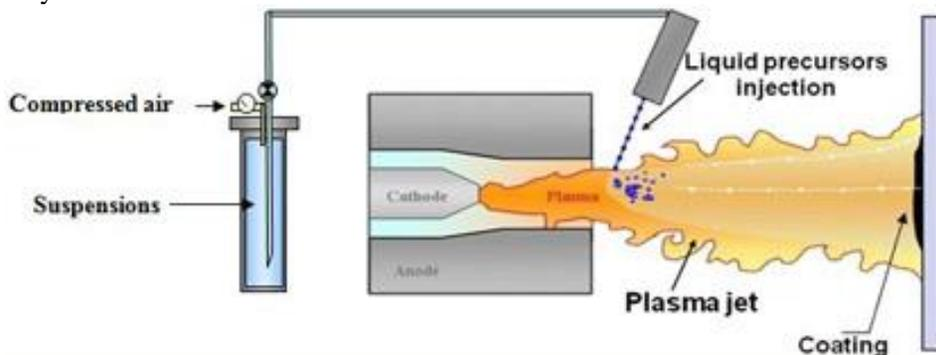
Fig. 2 Suspension plasma spray deposition [6]
