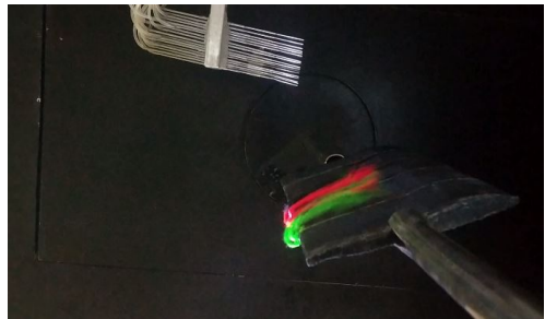
Figure 11: Flow reversal for Hybrid wing at AOA +18° and Re_c 120000
