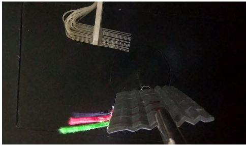
Figure 8: Tuft flow visualization for Corrugated wing at AOA+4 degree and Re_c 67000
