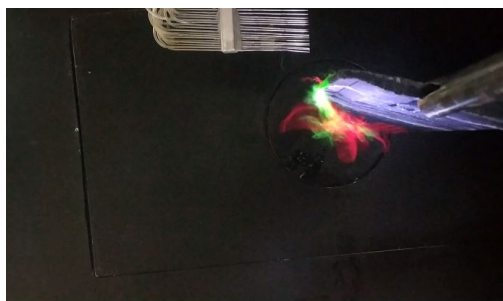
Figure 13: Flow reversal for Hybrid wing at -14^\circ AOA and Re_c 120000
