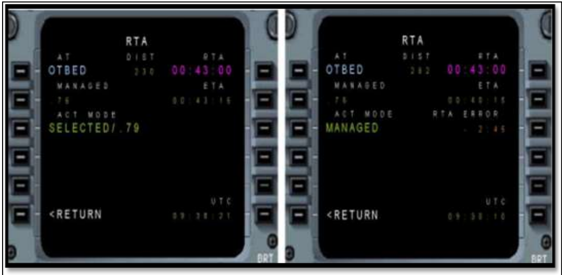
Figure 3. Visual explanation of the alarm system RTA ERROR
