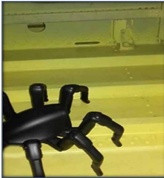
Fig. 6 – The hexapod mobile robot inside the central fuel tank of the Boeing 737-300 aircraft
