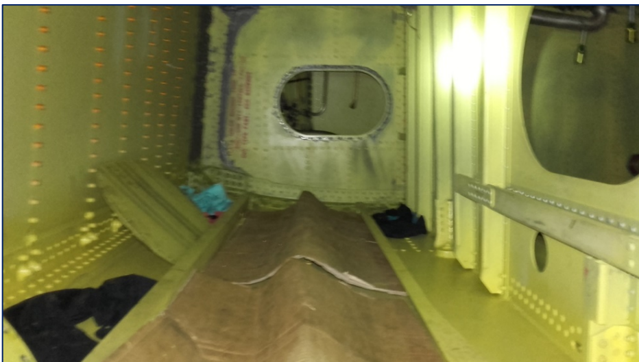
Fig. 4 – Removal of traces of kerosene left in the central fuel tank of the Boeing 737-300 aircraft
