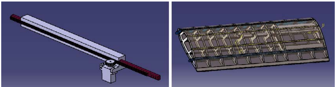
Fig. 2 Assembled wing with linear actuator
