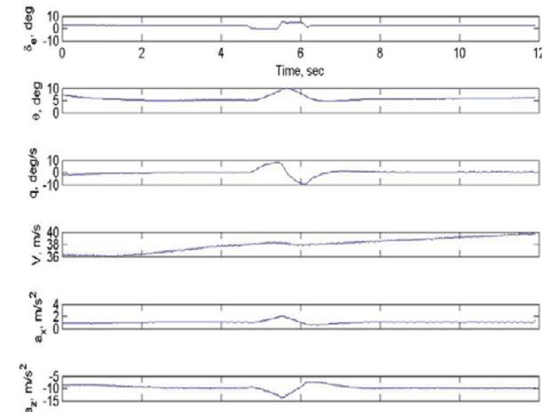
Fig. 3(b): Longitudinal Flight Data, HLD1
