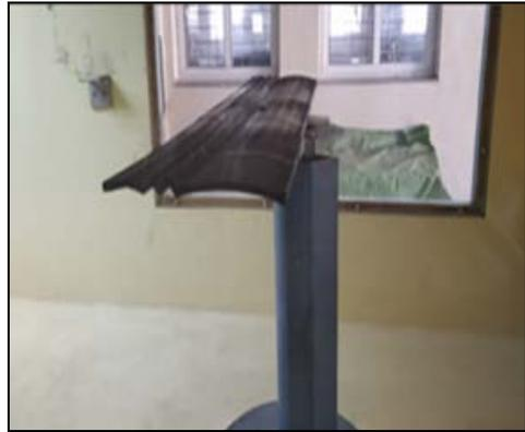
Fig. 12 Corrugated wing in wind tunnel
