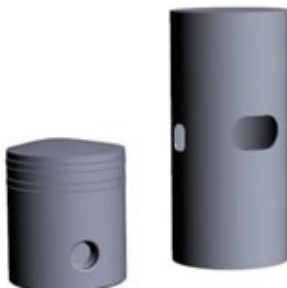
Figure 1: Model of the Engine Cylinder with elliptical shaped exhaust port
