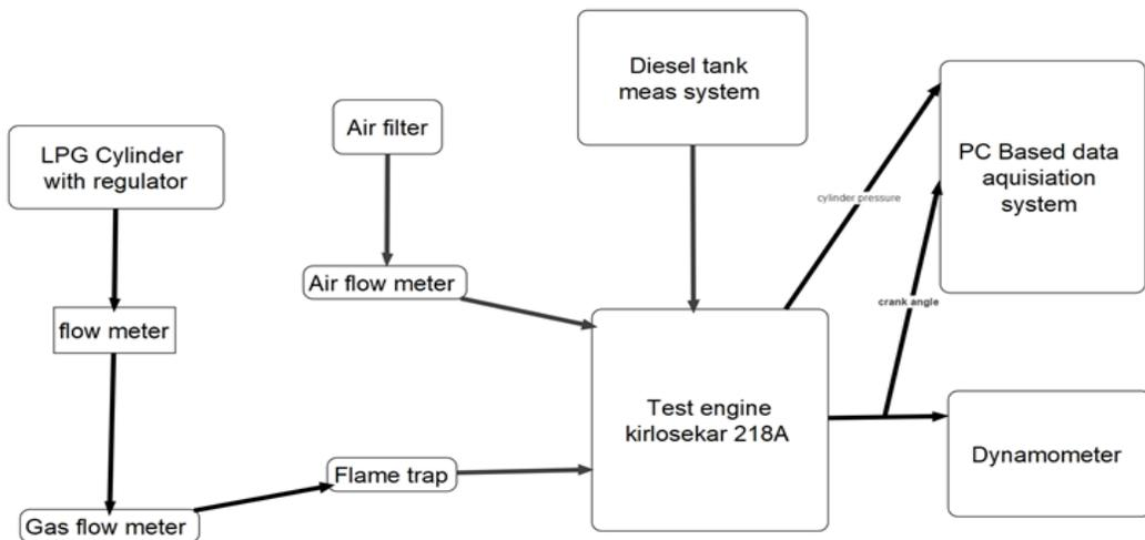
Fig. 1 The schematic diagram of the experimental setup
