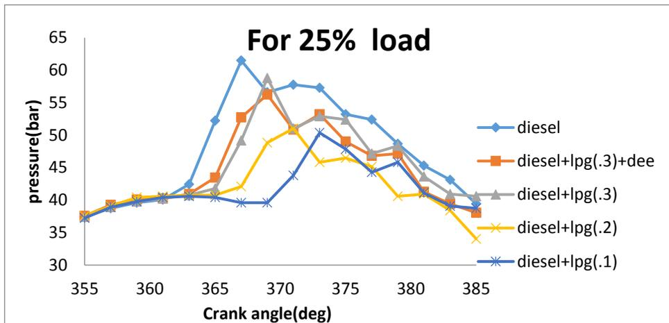
Fig. 3 Pressure-crank angle curves for 25% load for Diesel, Diesel + different Liquid petroleum product flow rates (0.118, 0.225 and 0.375 kg/h), 85% Diesel + 15% Diethyl ether + 0.375 kg/h of Liquid petroleum product
