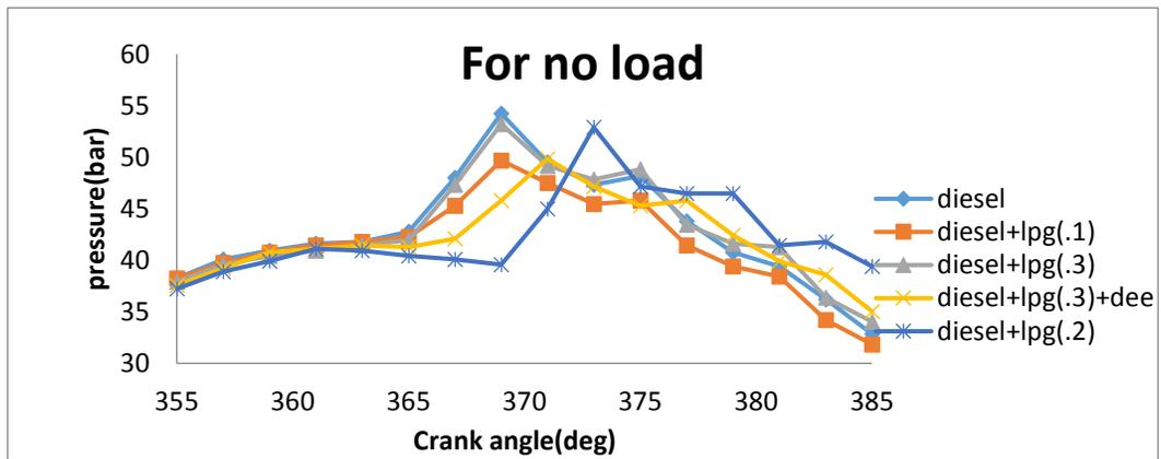
Fig. 2 Pressure-crank angle curves for no load for Diesel, Diesel + different Liquid petroleum product flow rates (0.118, 0.225 and 0.375 kg/h), 85% Diesel + 15% Diethyl ether + 0.375 kg/h of Liquid petroleum product
