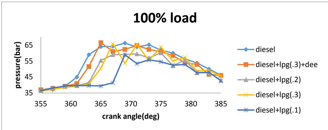
Fig. 6 Pressure-crank angle curves for 100% load for Diesel, Diesel + different Liquid petroleum product flow rates (0.118, 0.225 and 0.375 kg/h), 85% Diesel + 15% Diethyl ether + 0.375 kg/h of Liquid petroleum product
