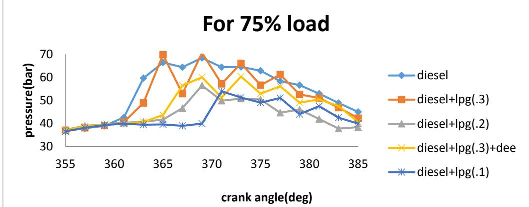
Fig. 5 Pressure-crank angle curves for 75% load for Diesel, Diesel + different Liquid petroleum product flow rates (0.118, 0.225 and 0.375 kg/h), 85% Diesel + 15% Diethyl ether + 0.375 kg/h of Liquid petroleum product
