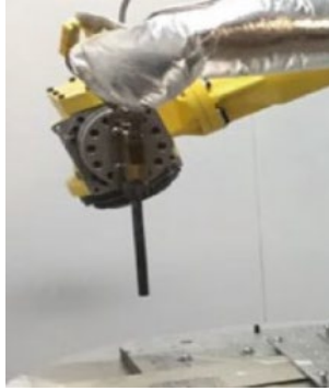
Figure 1. The spray nozzle of the Cold Spray installation mounted on the robotic arm
