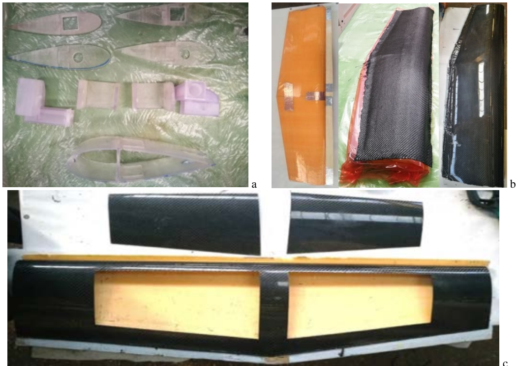
Fig. 11 – a) 3D printed parts using UV curing resin; b) Wing from extruded polystyrene cutted with hot wire; c) Access points for electronics
