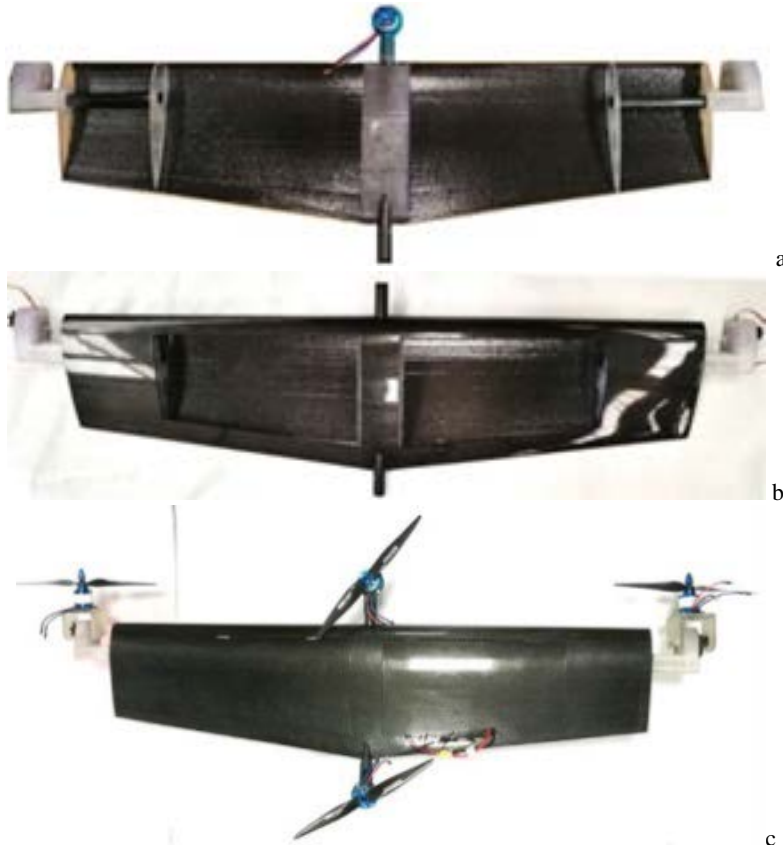
Fig. 12 – Three stages of the manufacturing process from left to right
