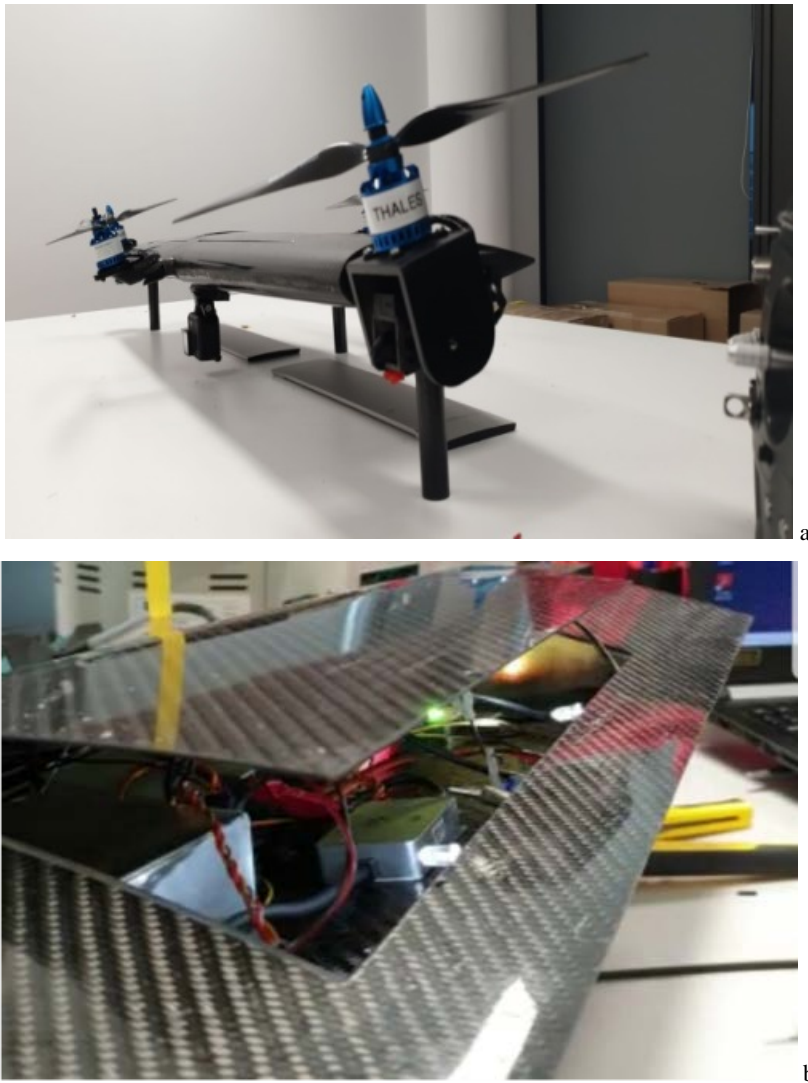
Fig. 13 – a) Final form of the UAV; b) Electronics hatch
