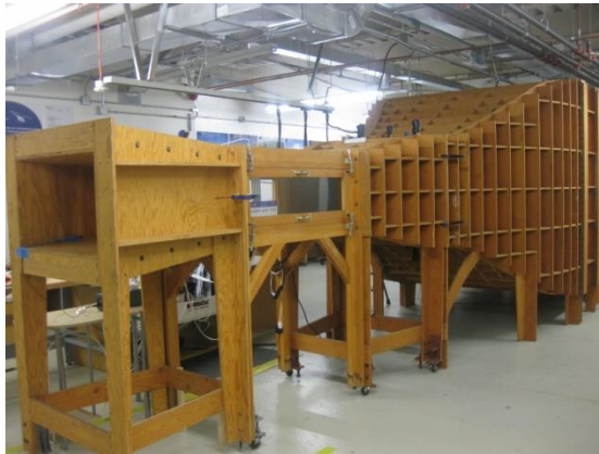
Figure 16. Price-Paidoussis Wind Tunnel
