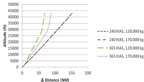
Figure 6. Variation of distance traveled with altitude in the descent for different speeds and weights
