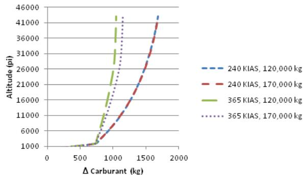
Figure 5. Variation of fuel burned with altitude in the descent phase for different speeds and weights
