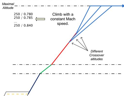
Figure 4. Speed calculation replication for 250 IAS to different Mach numbers
