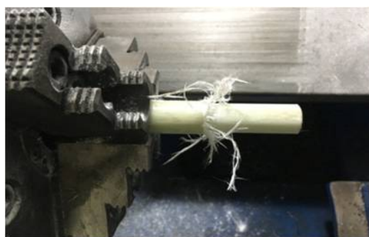
Fig. 4 – Turning of UD-GFRP Composite Jobs
