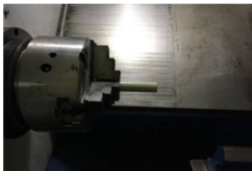
Fig. 3 – Setup of UD-GFRP Composite job
