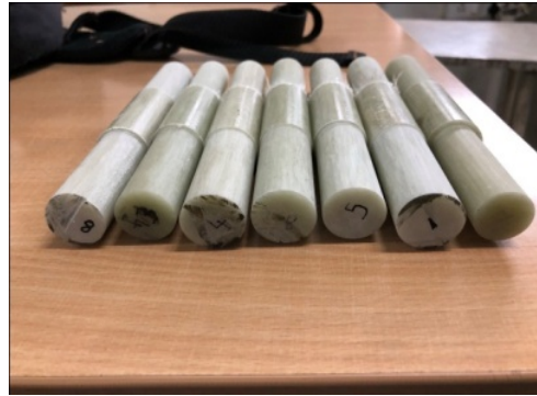
Fig. 6 – CNC turned composite parts
