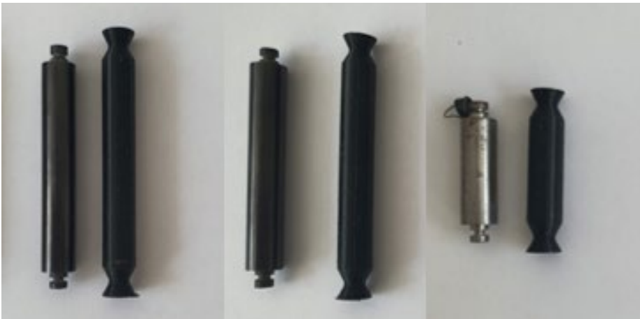
Figure 3. Loading bars from standard (S) and 3D printed (P) PLA material
