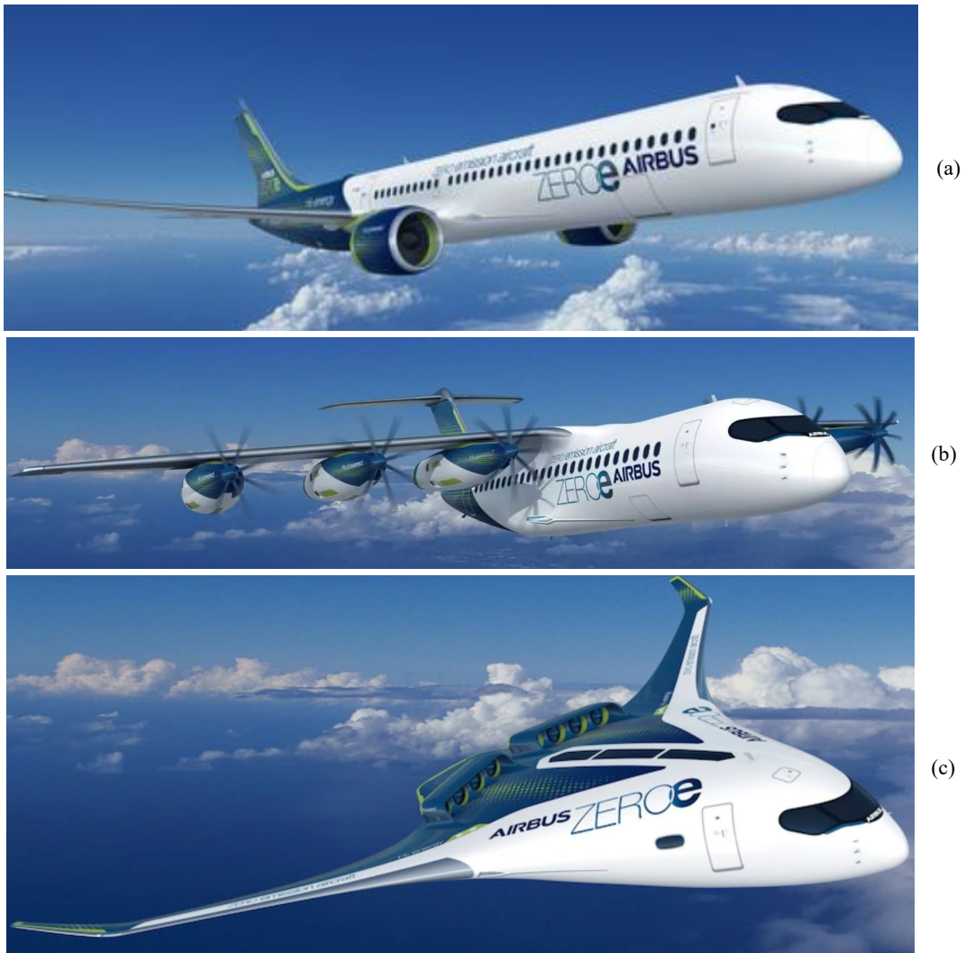
Fig. 2 AIRBUS ZEROe the three types of hybrid-hydrogen aircraft [12]
