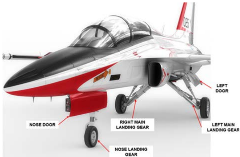
Fig. 1 Landing gear for a military training aircraft [6]
