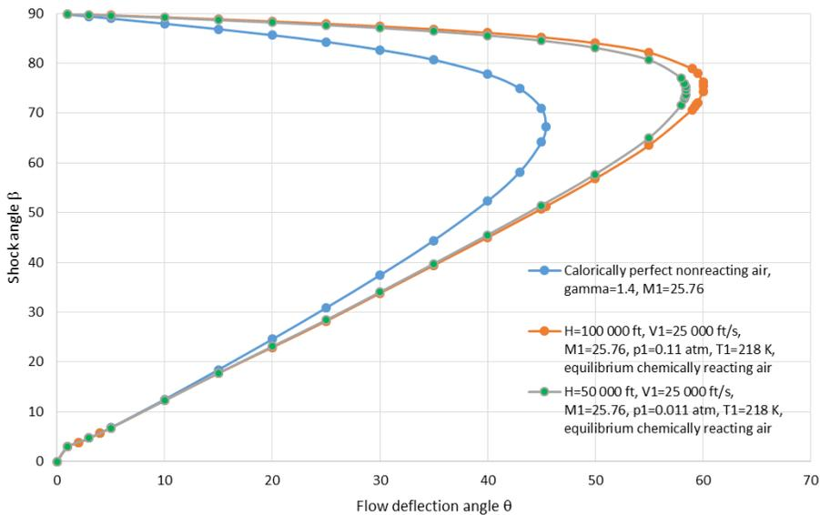
Fig. 1 – Influence of upstream pressure on oblique shock waves
