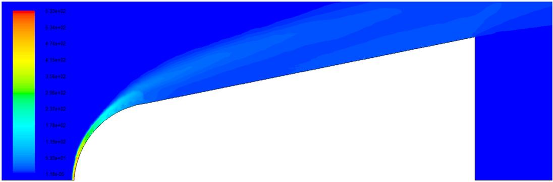
Fig. 3 – Pressure distribution for a reentry capsule,  $M_\infty = 20$ ,  $p_\infty = 0.8627$  Pa,  $c_{p,cr}$  are taken from [9] using ANSYS Fluent 15 [11] and AUSM scheme
