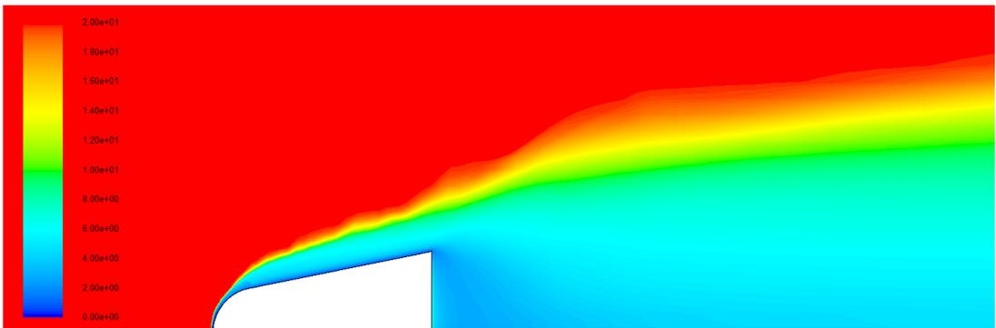
Fig. 2 – Mach number distribution for a reentry capsule,  $M_\infty = 20$ ,  $p_\infty = 0.8627\text{ Pa}$ ,  $c_{p\ cr}$  are taken from [9] using ANSYS Fluent 15 [11] and AUSM scheme
