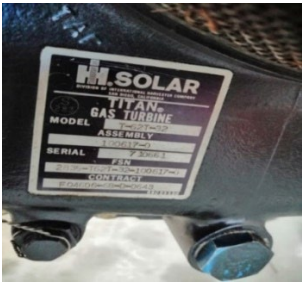
Fig. 9 - Identification plate of Solar turbo-shaft jet engine
