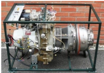
Fig. 7 - Turbo-shaft jet engine Solar installed on a GPU
