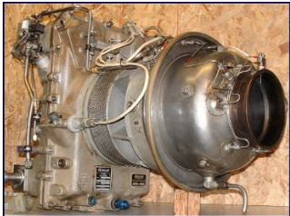
Fig. 8 - View of a Solar turbo-shaft jet engine
