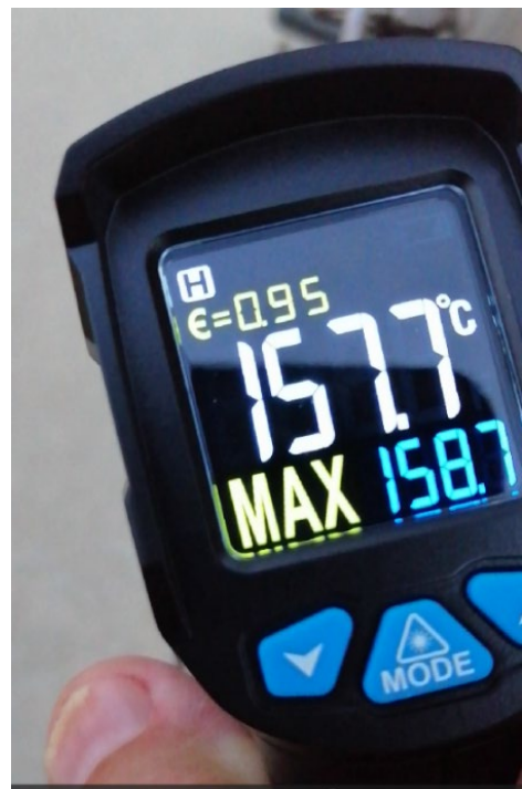
Fig. 11 - Hot case temperature for 40% power.
