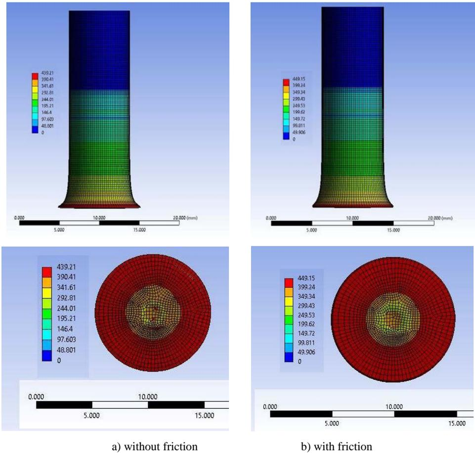
Figure 2. Lateral view of the projectile shape (up) and of the impacting surface (down), at time moment  $t=1 \times 10^{-5}$  s
