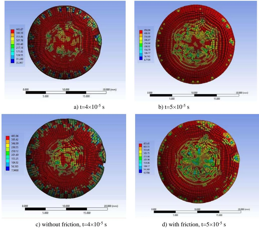
Figure 4. Von Mises stress distribution for important moments for mushroom development and failure
