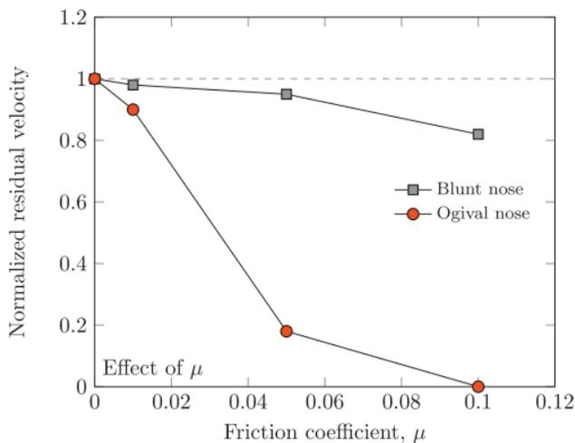
Figure 1. Simulation results of residual velocity, all parameters being constant, except for the friction coefficient.  $v_0=250\text{m/s}$  for the blunt projectile and  $v_0=350\text{m/s}$  for the ogival projectile using a yield-surface exponent  $a=2$  [7]
