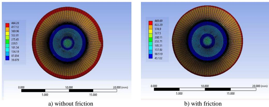
Figure 3. Top view (the target is invisible, here behind the projectile), at  $t=2 \times 10^{-5}$  s, von Mises stress distribution [MPa]
