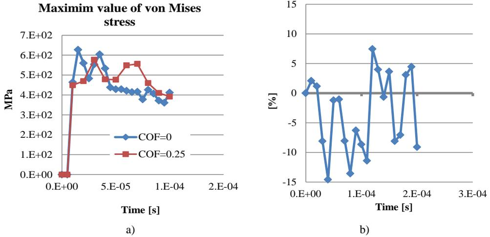
Figure 5. Maximum value of von Mises stress during the impact
