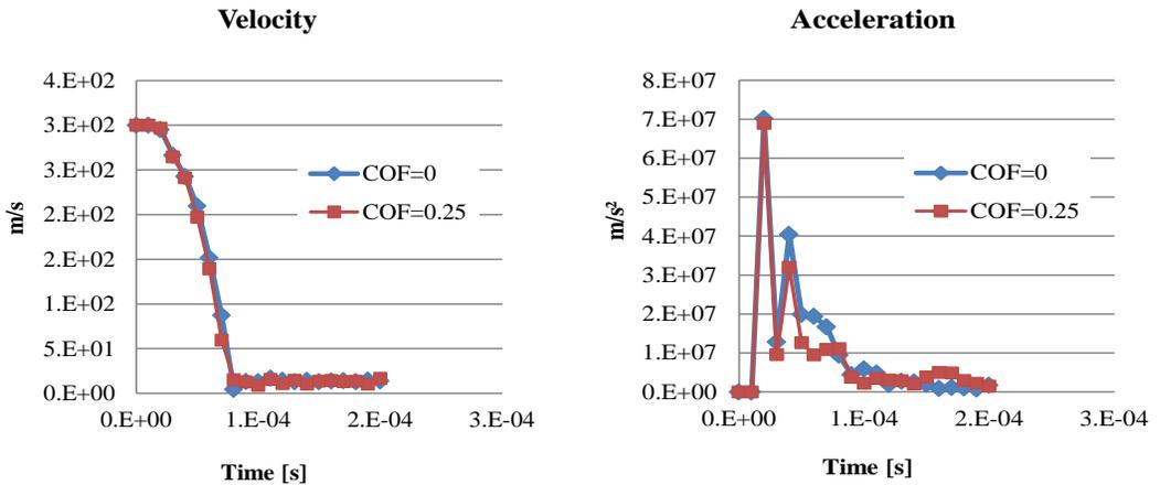
Figure 6. Velocity for the central point on the surface opposite to that in contact
