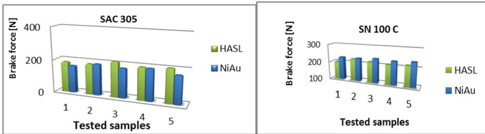
Fig. 3 Brake force variation for SAC 305 and SN 100C solder pastes
