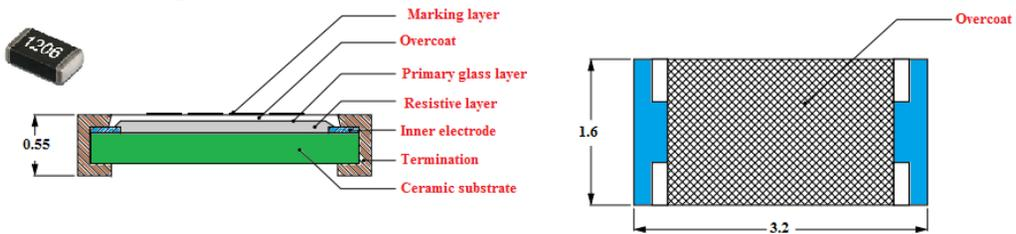
Fig. 1 Chip resistor (1206)
