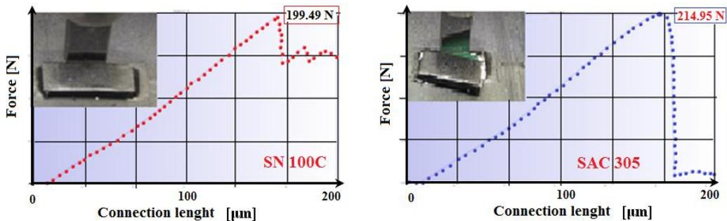
Fig. 4 Force variation for SN 100 C (ductile fracture) and SAC 305 (brittle fracture)
