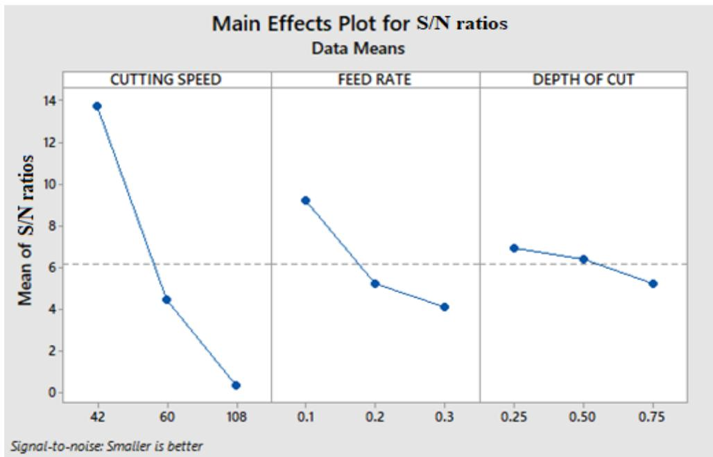
Fig. 6: Plots for mean S/N ratios for Material Removal Rate
