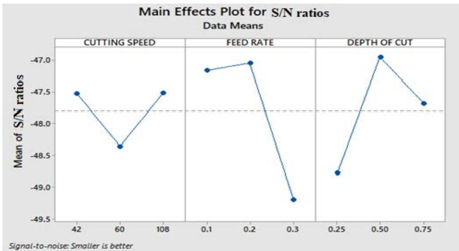
Fig. 4: Plots for mean S/N ratios for Mean Cutting force
