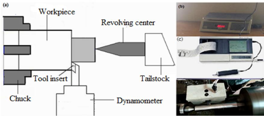
Fig. 1: Experimental setup (a) Schematic layout of experimental setup (b) photograph of weighing scale device to measure weight(c) photograph of surface roughness tester (d) photograph of experimental setup showing dynamometer attached to tool
