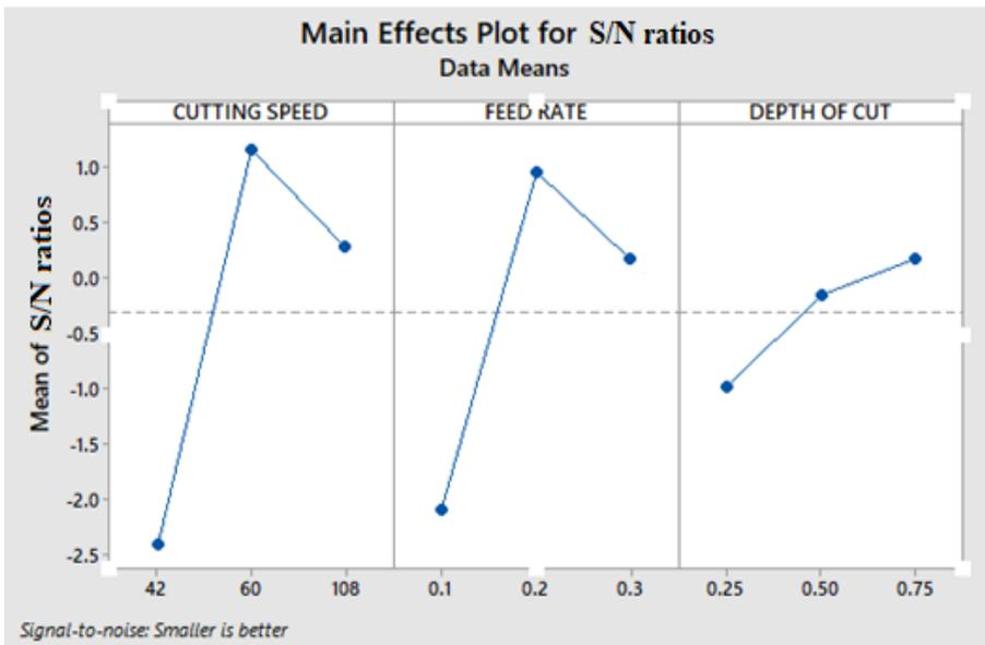
Fig. 5: Plots for mean S/N ratios for Surface Roughness
