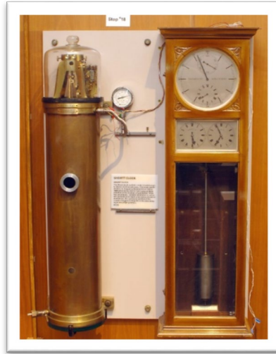
Figure 1. The Shortt-Synchronome No 32 free pendulum high precision time reference, used as the US Frequency Standard from 1924 to 1929. The master pendulum is encased in a vacuum cylinder to the left, and the slave clock has electric contacts to distribute 1PPS (one pulse per second) standard scientific time signals. It was subsequently used to determine the gravitational constant by Heyl [14]. The basic principle is behind any PLL oscillator of today and its “asynchronous synchronization” technology, called the “hit and miss synchronizer” is the basis of a proper GPS-DO (GPS disciplined oscillator)
