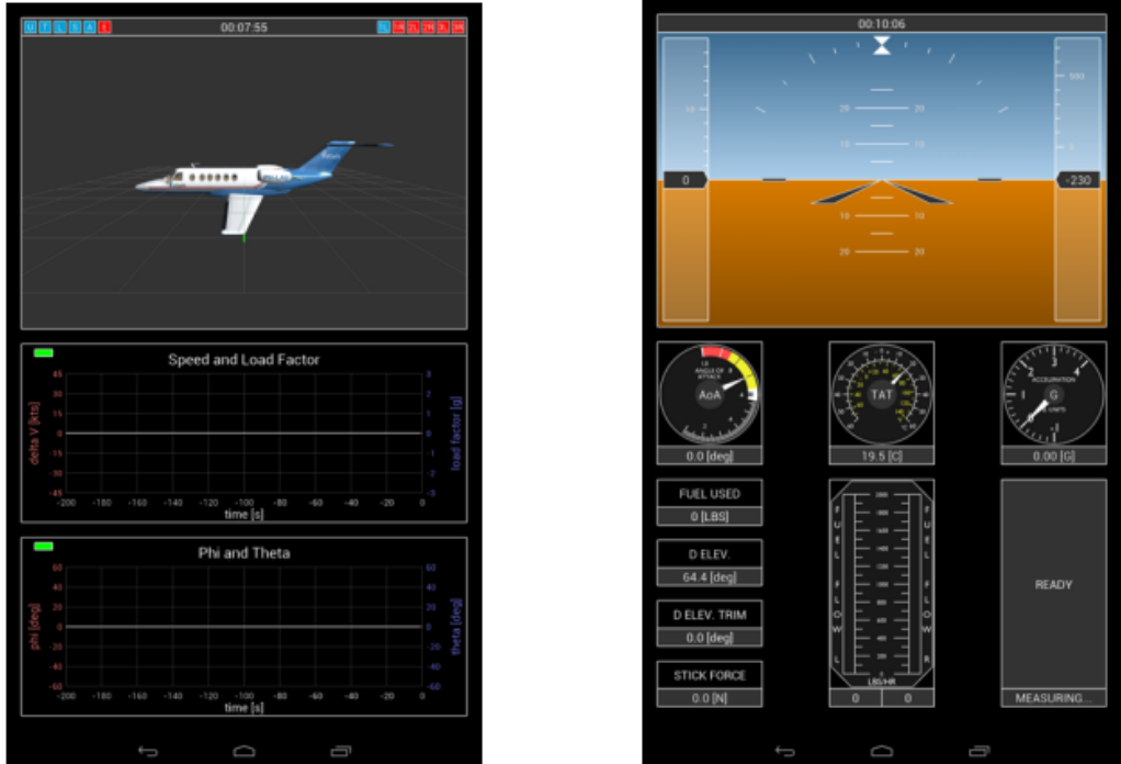
Figure 1. The INDI cockpit instruments/ displays developed on Cessna Citation Aircraft as fly-by-wire technology (int' Veld et. al., 2018)
