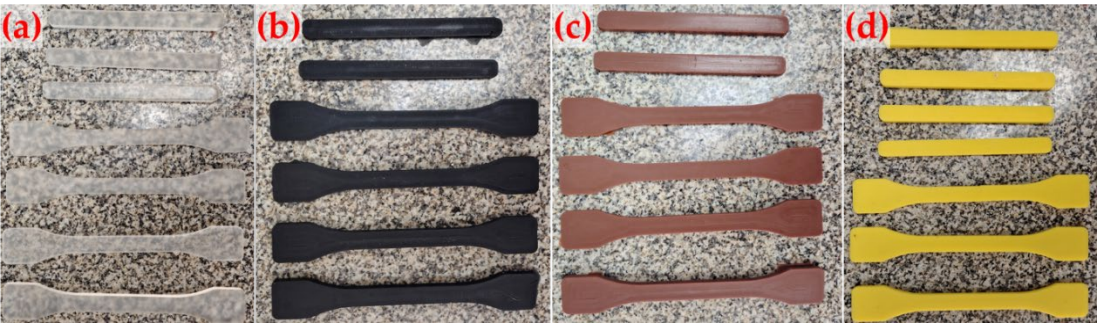
Fig. 2 – The obtained nanocomposites: (a) Control Epoxy, (b) Epoxy+1%CNT-Ni, (c) Epoxy+1%BaFe 12 O 19 , (d) Epoxy+1%Bi 2 O 3
