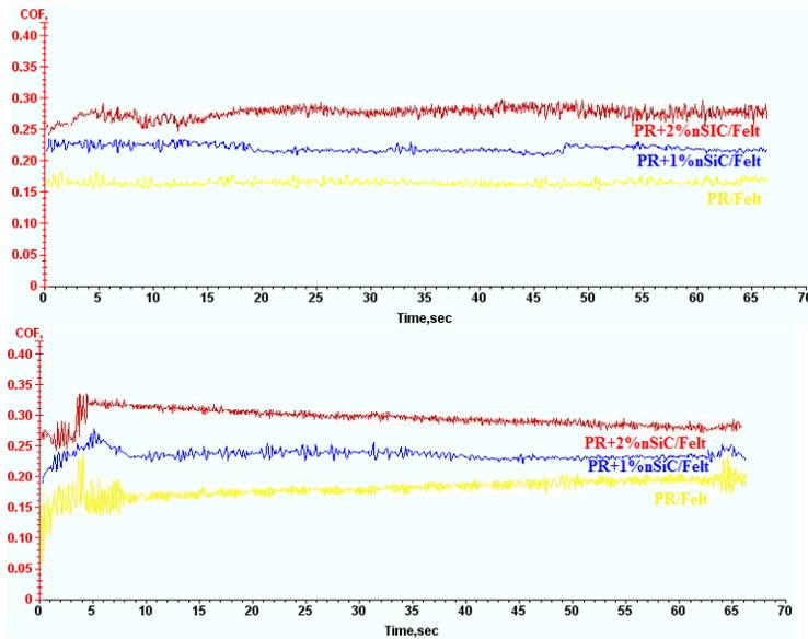
Friction coefficient of PR/nSiC/Felt measured at 1000 rpm
