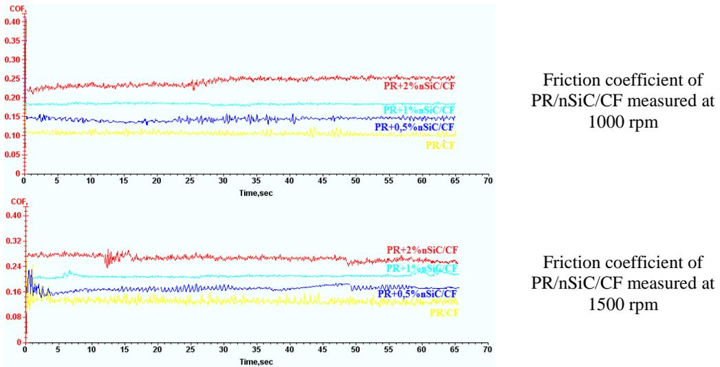
Fig. 4 Friction coefficient of PR/nSiC/CF
