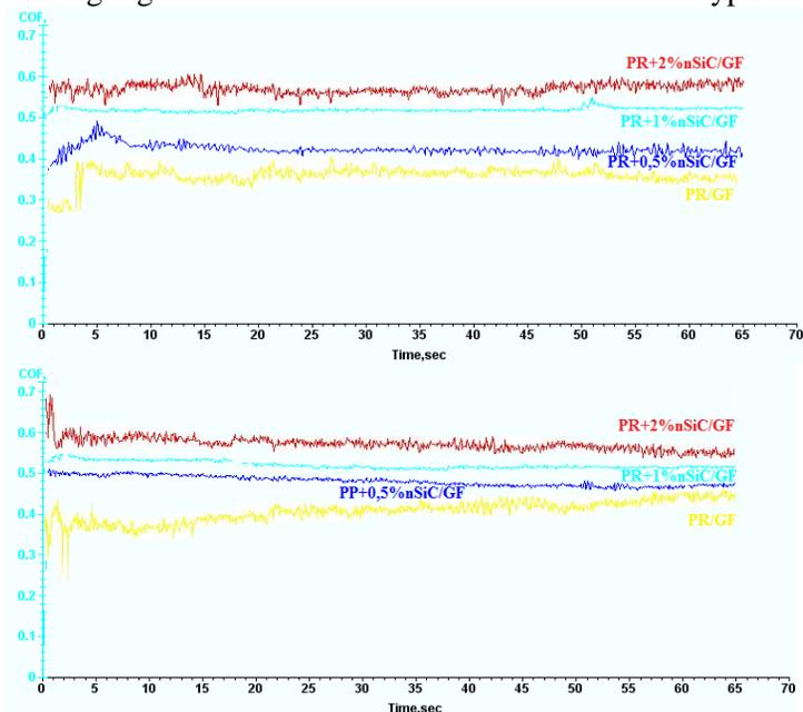
Friction coefficient of PR/nSiC/GF measured at 1000 rpm
