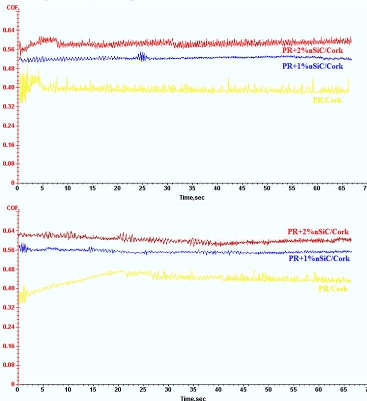
Friction coefficient of PR/nSiC/Cork measured at 1000 rpm
