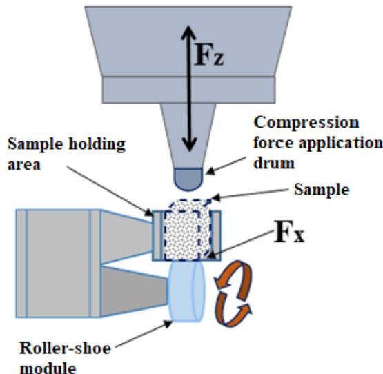
Fig. 1 Diagram of the tribological installation with the roller-shoe mode [1]
