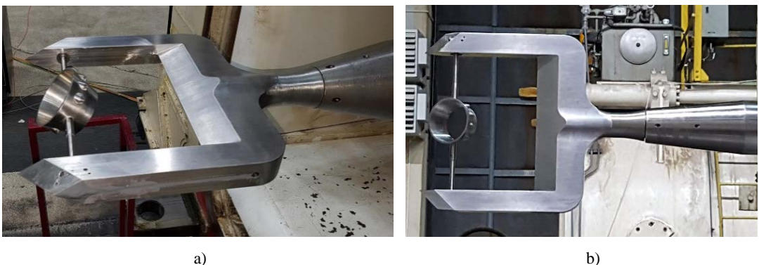
Figure 2. FTT model installed on the rig, a) roll angle 0 deg, b) roll angle 90 deg
