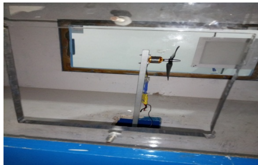
Fig. 2 - Single Propeller mounted in the wind tunnel load cell
