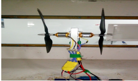
Fig. 3 - Twin Propeller mounted in the wind tunnel load cell
