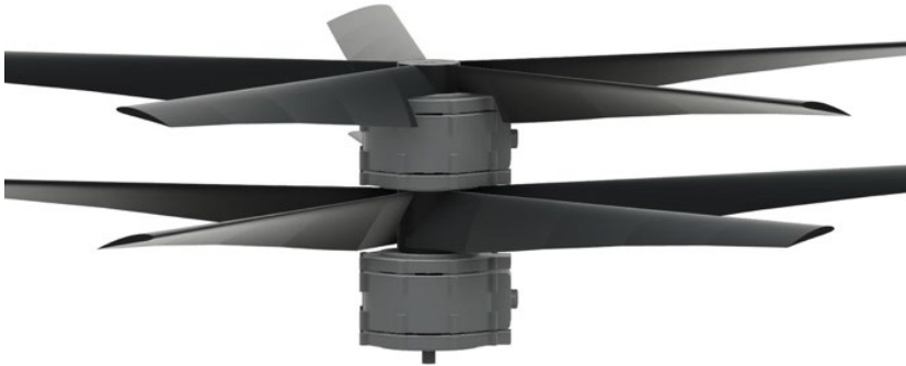
Figure 14 – Coaxial rotor, twisted blade airfoil
