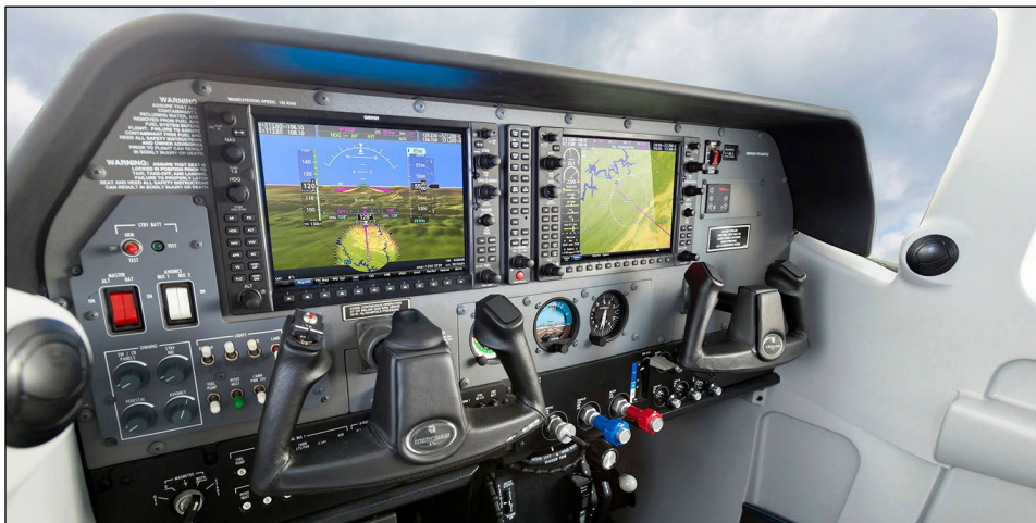
Figure 11. GARMIN G1000 NXi flight deck installed in a small GA aircraft [11]
