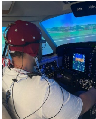
Fig. 2 – Pilot wearing BN-EEGCAP-SYS, BN-BIOSHIRT and Tobii Pro Glasses 2
