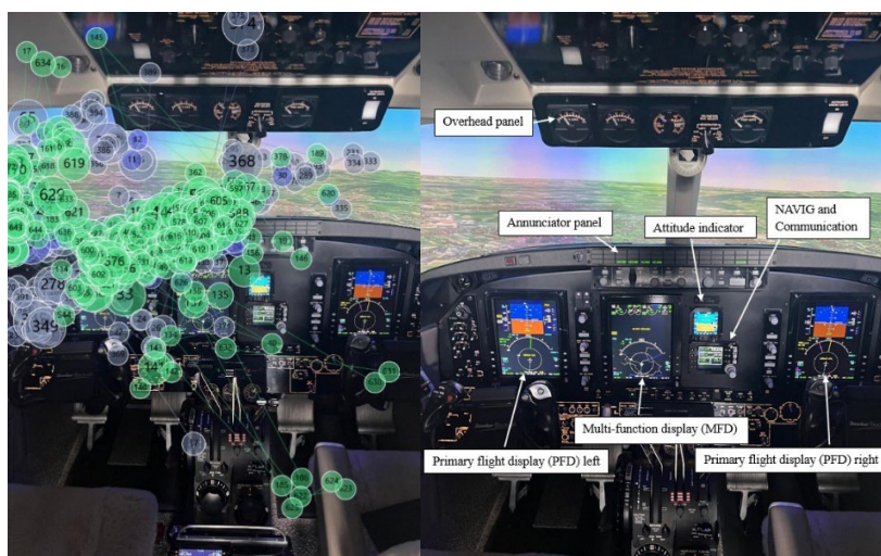
Fig. 12 – Gaze plot illustrating visual attention distribution across the three simulated flight scenarios: Flight 1 (grey), Flight 2 (green), Flight 3 (blue) – alongside the flight deck layout for Beechcraft King Air C90 Flight simulator
