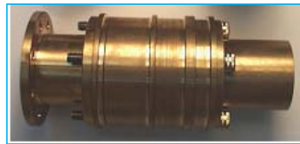
Fig. 8 Subscale test motor with variable length chamber
